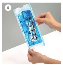
Allow the ink take effect on every seal seam for c. 5 seconds. Check all seal seams for leaks.
